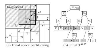
Fig. 9 Final  $T^{KD}$  partitioning and structure
